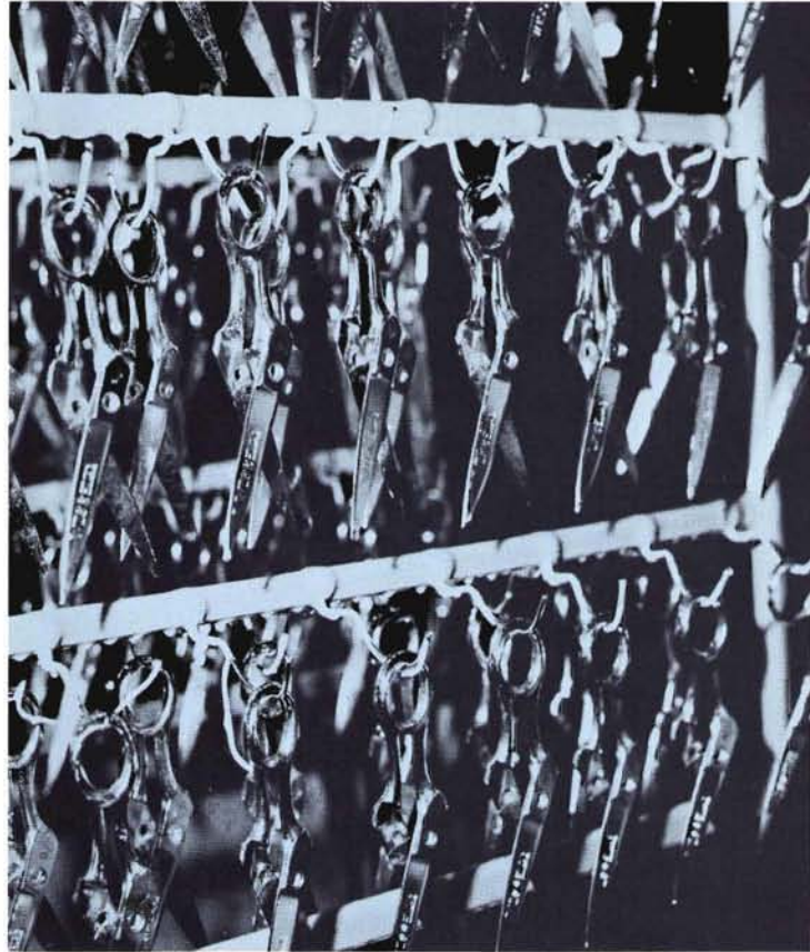
—Before final assembly, blade and handle are fully nickel plated to prevent rust, and to provide a quality product that will retain its attractive appearance and insure high performance after extensive use.
